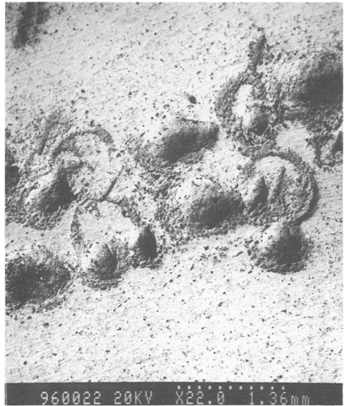
FIG. 4—SEM photomicrograph showing second and third digit of restored serial number.
