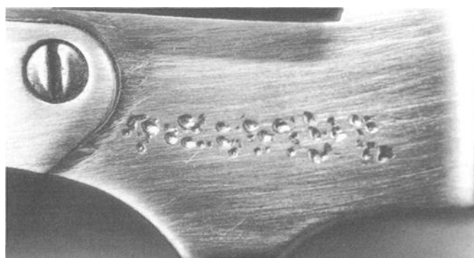
FIG. 1—Photograph showing area of obliterated serial number prior to restoration.
