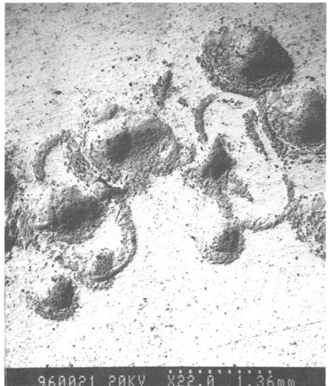
FIG. 5—SEM photomicrograph showing fourth and fifth digit of restored serial number.
