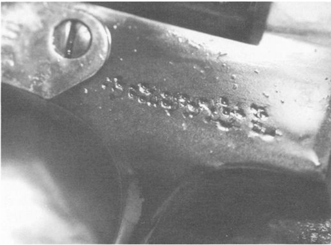
FIG. 2—Photograph showing area of obliterated serial number following restoration with Fry's etchant.
